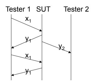
The tester at port 1 observes x<sub>1</sub>y<sub>1</sub>x<sub>1</sub>y<sub>1</sub> and the tester at port 2 observes y<sub>2</sub> only.
