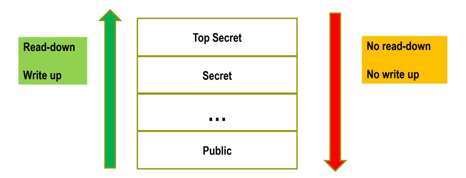
Data can flow only upwards
